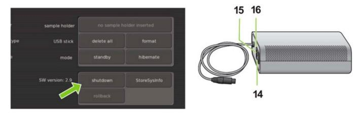
4. You can now completely shut down your system by pushing the 0/I button (14) on the power supply.
